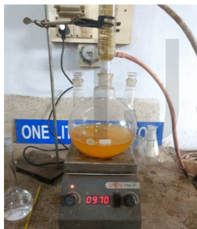
Fig. 6: 3-Neck Flask with uniform heating and stirring
